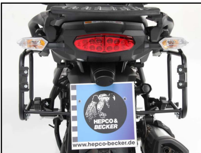
Width of the side carrier 52 cm plus case width
