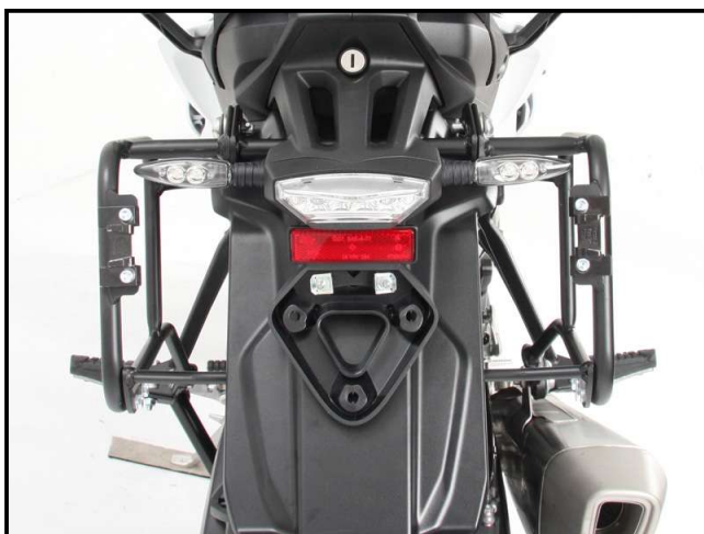
Width of the side carrier 40 cm plus case width
