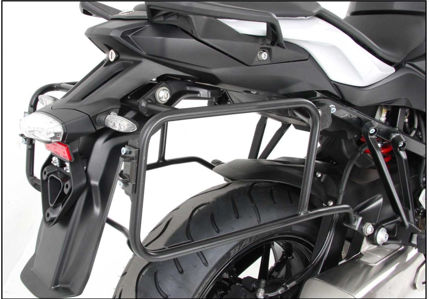
Width of the side carrier 40 cm plus case width
