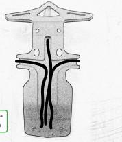
Run wires neatly down the channel in both parts ensuring they do not get trapped or squashed
