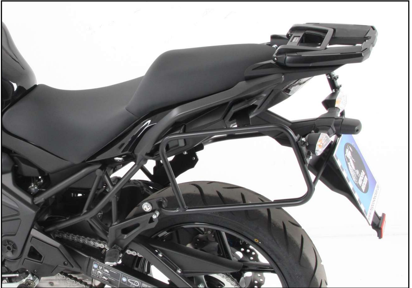
Width of the side carrier 47,5 cm plus case width
