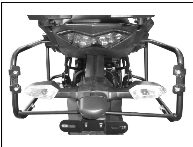
Width of the side carrier 47,5 cm plus case width
