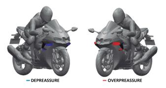
Due to its angles and frontal surface, it creates an overpressure on the top of the spoiler. The turbulance create below, generates a difference of pressure between the upper and lower part of the spoiler. Which ultimately generates the aerodynamic downforce.
