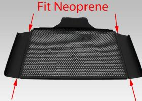
3. Remove the upper 2 locating bolts. Hook the radiator guard on the lower edge then secure the radiator in position using the original bolts.
