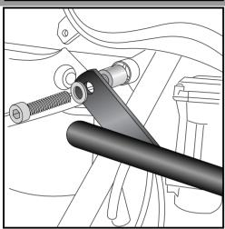
Fastening of the engine guard top left + right:
