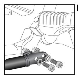
2 Fastening of the engine guard bottom left + right:
