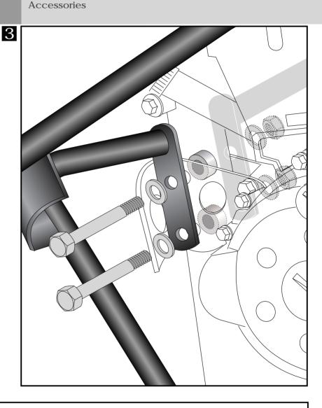
Control all screw connections after the assembling for tightness! Please notice our enclosed service information.
