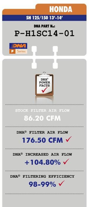
AIR FLOW DATA MEASURED WITH DNA'S ROTRONICS FLOWSCAN COMPUTERIZED FLOWBENCH
