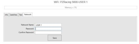
From the software, in the Network tab, it is possible to change the last part of the network name (USER 1) and the password. Once modified it will be necessary to close the RacePro program, turn off and on the GPS receiver.
