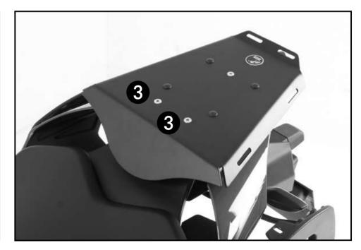
Seal up the 4 holes not in use with sealing plugs. Fixing the SPORTRACK onto the motorbike is the same as fixing a pillion seat. Please check that the SPORTRACK is securely fitted before driving.
