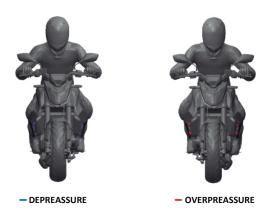
Due to its angles and frontal surface, it creates an overpressure on the top of the spoiler. The turbulance create below, generates a difference of pressure between the upper and lower part of the spoiler. Which ultimately generates the aerodynamic downforce.
